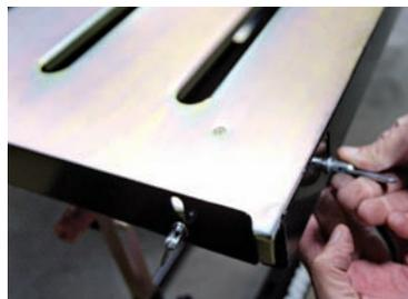
Also cool are the adjustable fences. You can raise them up to keep stuff from rolling off the table. They are held in place with easy-to-turn flag bolts. Start to finish, assembly took less than 30 minutes and we were up and welding.
