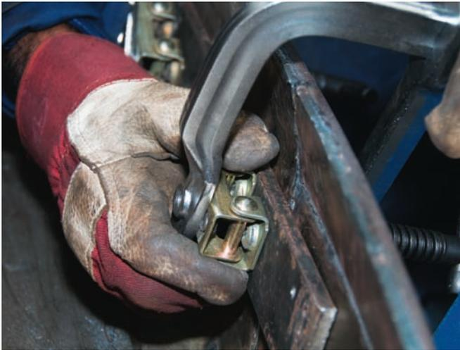
V blocks spread the load well and are less prone to slip on uneven surfaces.
