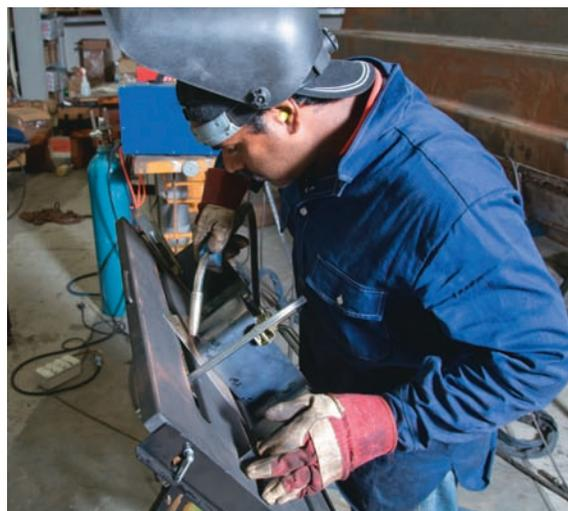
**The table tilts to allow access to the work at all angles.**
