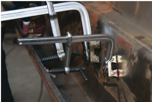
Clamps used as spreaders proved surprisingly effective and far easier than the two-tonne hydraulic jacks we had tried to manoeuvre in here.
