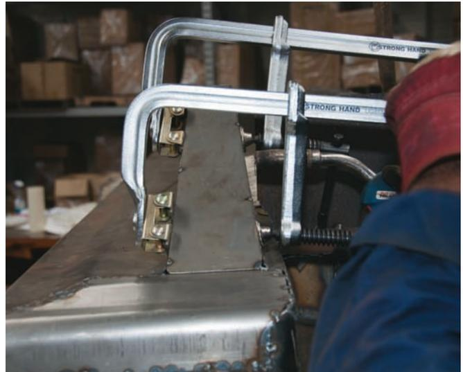
Strong Hand 4-in-1 clamps attach to uneven surfaces.
